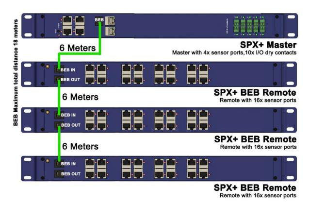
As shown in the diagram above, you can mount each BEB in the 1U configuration and daisy chain them using the BEB connection ports. The BEB units must be connected one at a time, not all at once. When disconnecting and then re-connecting the BEB to a different SPX+ base unit you will need to reset the BEB using the reset button on the BEB unit.
